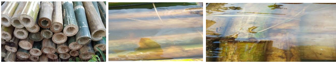
(h) Kiln Drying (i) Treated with Seawater (j) Treated with seawater +Mango Polyphenol
