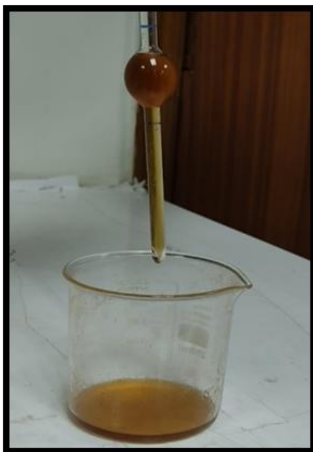
Figure 2: Surface Tension determination by Stalagmometer
