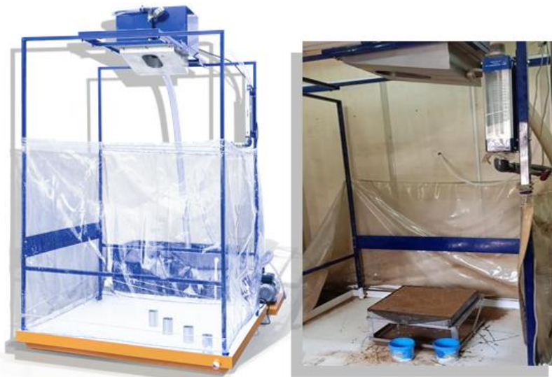
Fig 2: FEL3 Rainfall Simulator lab for water erosion test in Soil Erosion Unit, Desert Research Center (DRC)
