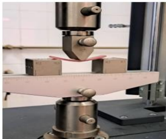
Figure 2: The 3-point bending test using Metrotech MTE-25 universal testing machine
