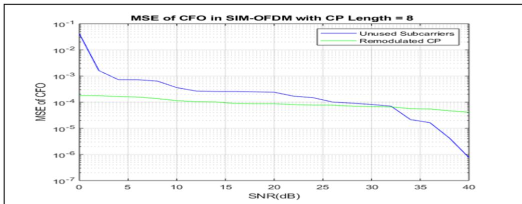
**Fig. 5: Performance plot of SIM-OFDM: MSE of offset estimation Vs. Varying SNR**
