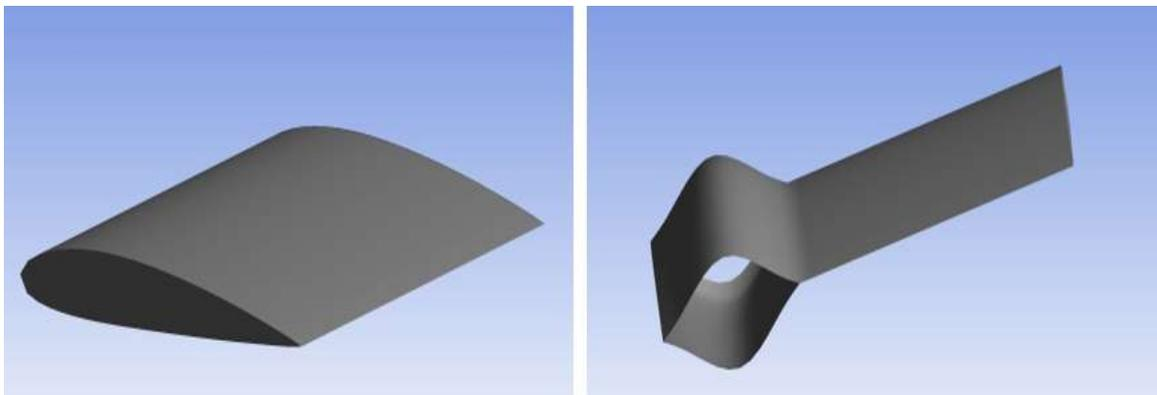
**Fig 3: Naca Profile 2415 with and without Winglet**
