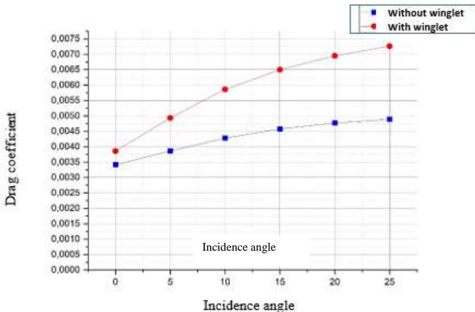
**Fig 8: Drag coefficient**
