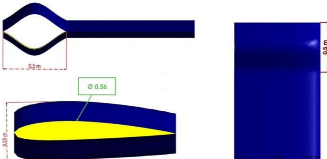
**Fig 2: Spiroid Winglet Dimensions**
