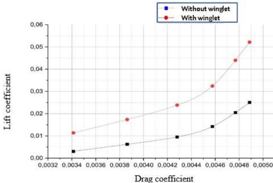
**Fig 9: Comparison of Lift and Drag Coefficients**
