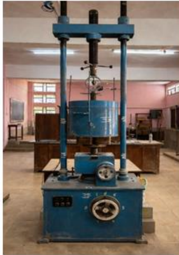
Fig 4: Loading Frame for static loading
